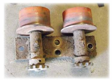
Used bushing, to be rebuilt
