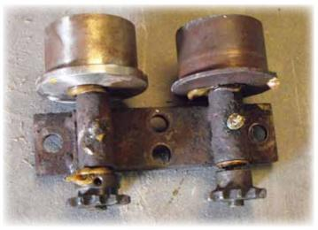
Rebuilt bushing, note the gold-colored Almaplex 1299 lubricant
